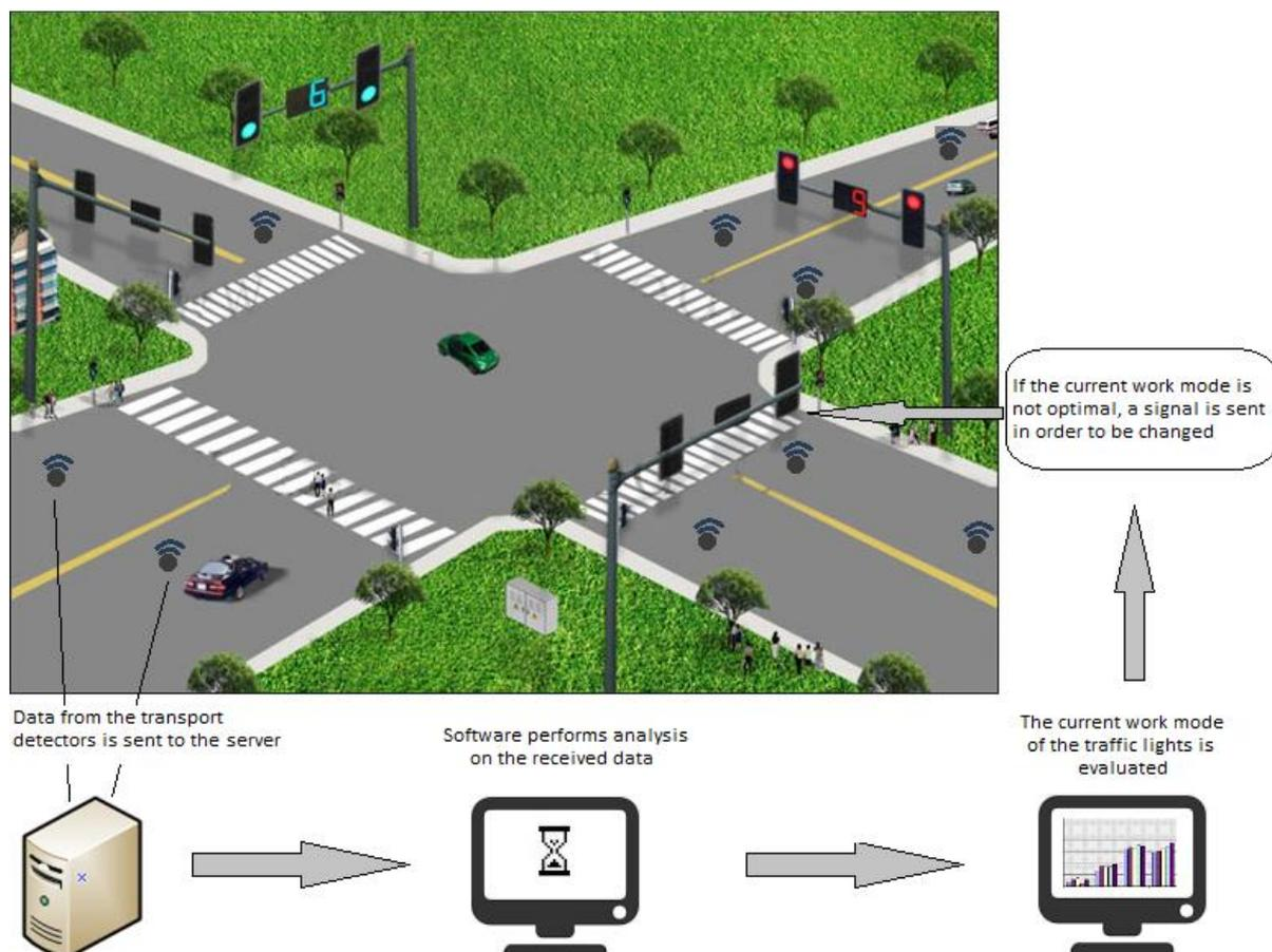
**Figure 3.** A scheme of how the traffic light control module functions
